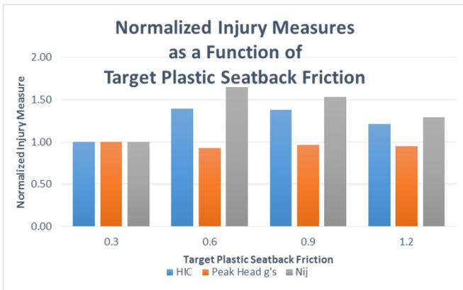
Figure 3. Results from PE1 test series varying target seat to ATD friction levels
