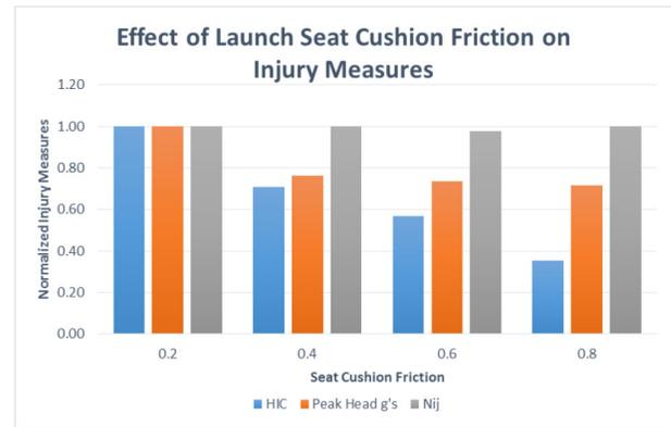
Figure 5. Effects of launch seat friction on injury measures
