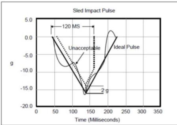
Figure 1. Frontal sled impact pulse requirement from 14 CFR 25.
