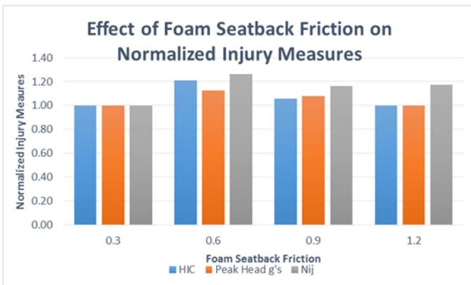
Figure 4. Injury measures obtained with increasing target seat frictions
