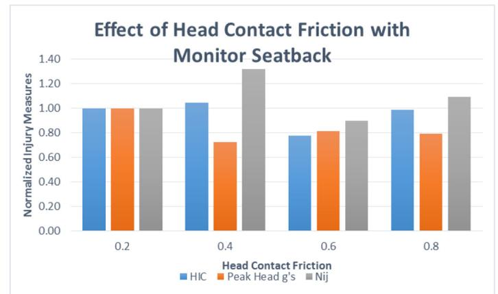
Figure 2. Effect of head contact friction with monitor seatback
